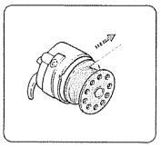
making sure thread feeds clock- as shown. wise and is coming from bobbin as shown.
